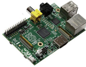
Figure 5. Carte Raspberry PI B+® (photo : Raspberry.org).
